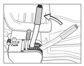
2. Rider 11 and Rider 11 Bio: Pull back the throttle lever and shift the gear lever into neutral "N". Turn the ignition key to the "STOP" position.
